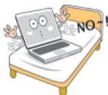
**Do not use the laptop on top of carpet, blanket or bed. Also, do not put the adapter under the blanket.**
